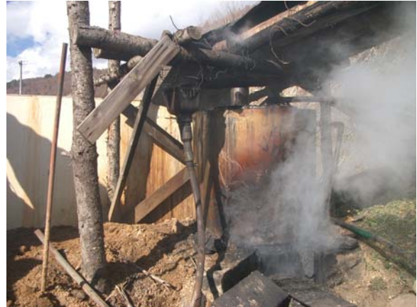
1-8 Water cooling Mokusaku liquification
