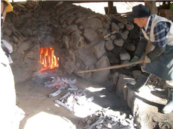
1-7 Charcoal kiln (built by stone)
